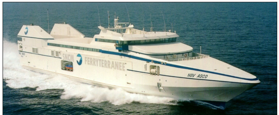
High Speed Ferry with ND Active T-Foil, Fins and Trim Tabs Integrated RCS
