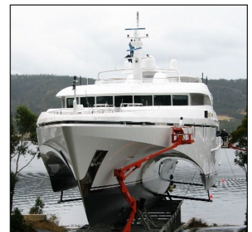
Trimaran with ND Active Lifting Foils
