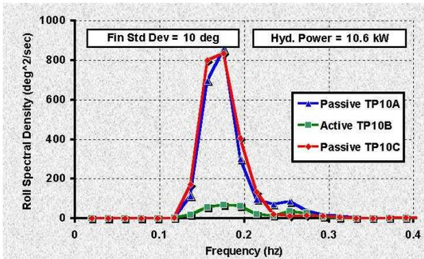
The Roll Spectral Density (RSD) graph on the left is a measure of roll energy. The x-axis represents the wave encounter frequency. Each curve peaks at the vessel's natural frequency (period) while far outside the vessel's natural period little roll energy is present. The Passive (Off) recordings (blue and red traces) were made immediately before and after the Active (On) recording (green trace). The duration of each trace was statistically appropriate.
