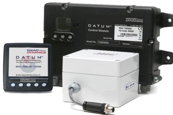
Additionally, the stabilizer system may be operated in the 'AtSpeed' (underway) or 'Adaptive' (self-learning) mode. The ability of the DATUM to self-learn and automatically adapt to its operating environment results in *continuously optimized* fin commands and astonishingly superior roll reduction performance.
