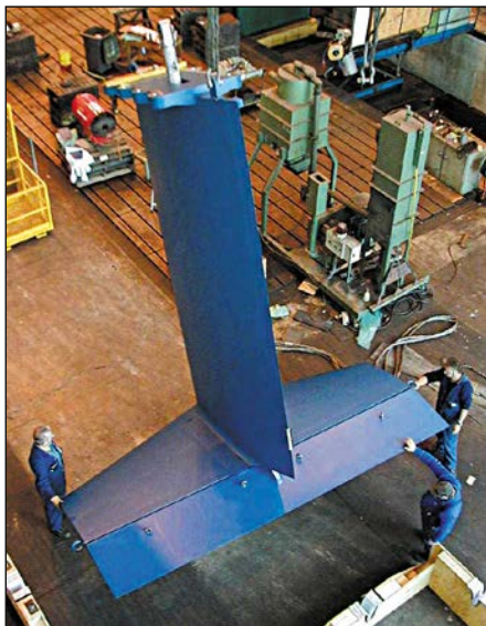
ND Retractable T-Foils can be stowed in calm conditions, are strike tolerant, and can be maintained and serviced in the water.
