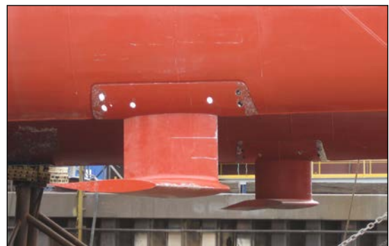
57m FBMA Catamaran with dual ND flapped T-Foils.
